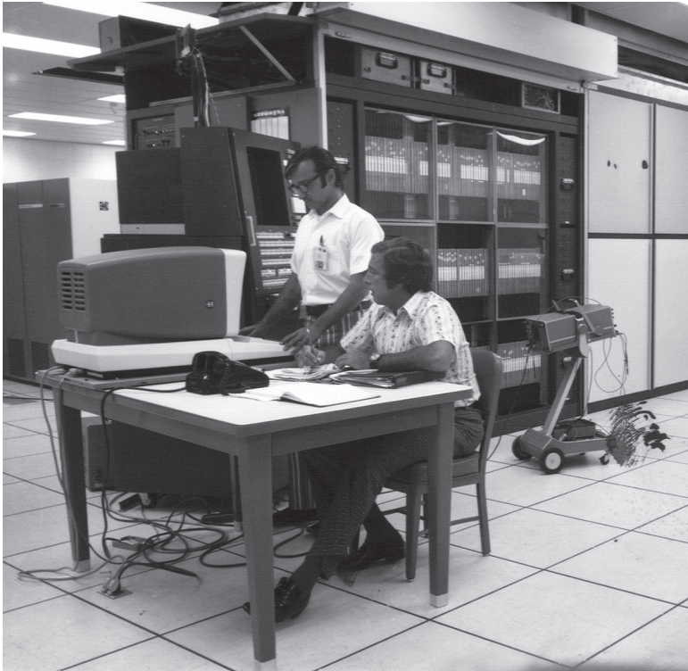
FIGURE 6.15.1 The Illiac IV control unit followed by its 64 processing elements. It was perhaps the most infamous of supercomputers. The project started in 1965 and ran its first real application in 1976. The 64 processors used a 13-MHz clock, and their combined main memory size was 1 MB: 64 \times 16 KB. The Illiac IV was the first machine to teach us that software for parallel machines dominates hardware issues. Photo courtesy of NASA Ames Research Center.
